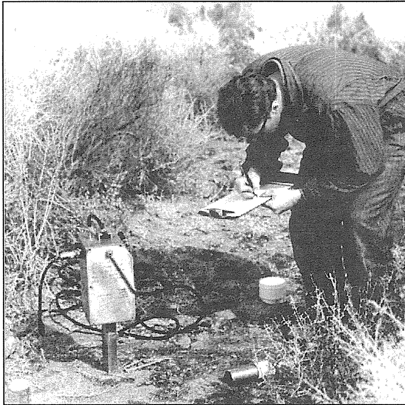
ICWD researcher Brian Cashore uses a neutron probe, a more accurate, efficient gauge of Owens Valley soil water conditions.
