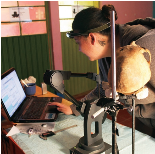
Figure 7. Kassie Sugimoto (MA North Carolina State University) configures a microscribe, an instrument that allows the creation of a quantifiable, three-dimensional digital image. Kassie is testing the hypothesis that childhood illness causes facial asymmetry in adults.
