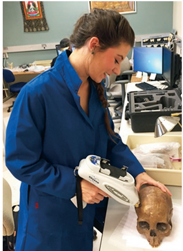
Figure 6. Ashleigh Lopes (BA UC Santa Barbara) uses a portable X-ray fluorescence Tracer (a “reverse recipe instrument”) to detect the presence of toxic metals in the bones of ancient copper miners.
