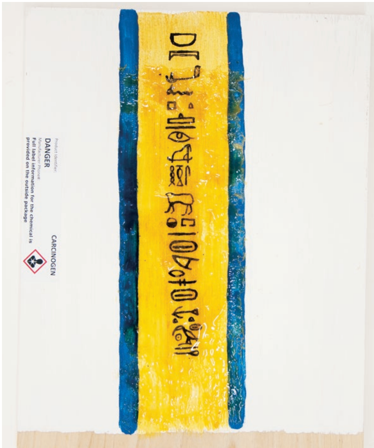
Figure 6. A test board with preparation layers, a painted background, a hieroglyphic inscription, and final varnish layers.
