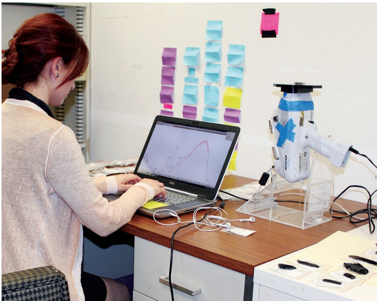
Figure 2. Kristine Martirosyan-Olshansky analyzes obsidian artifacts from California with a Bruker pXRF instrument.
