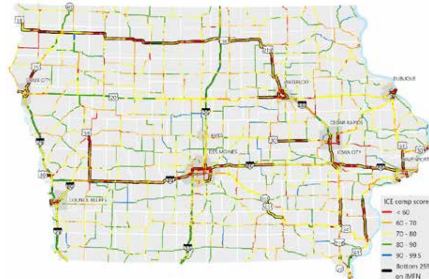
Figure 2.10: Infrastructure Condition Evaluation rating
