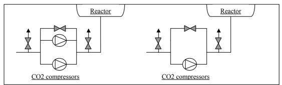
Figure 3: CO2 compressors at 100% load (left) and at 50% load (right)
