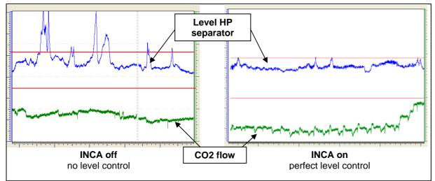
Figure 4: HP separator level with INCA turned off (l) and INCA turned on (r)
