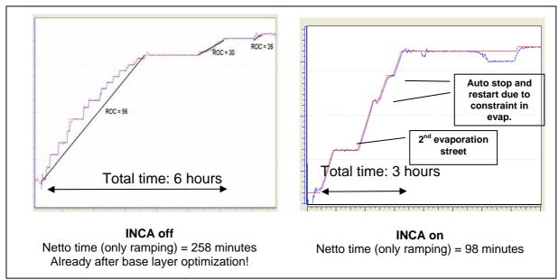
Figure 7: Ramping of CO2 flow from 50% to 100% load with INCA turned off (l) and INCA turned on (r)
