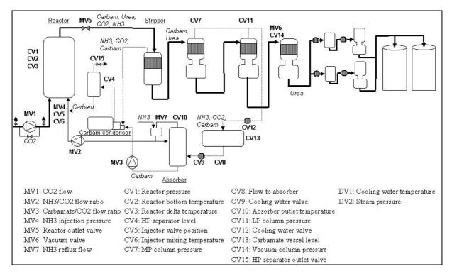
Figure 1: Schematic overview of a urea plant with INCA model variables
