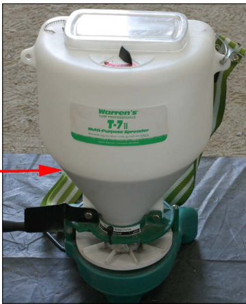
Photo 5. Keep the spreader at least 25% full, as shown by the arrow.
