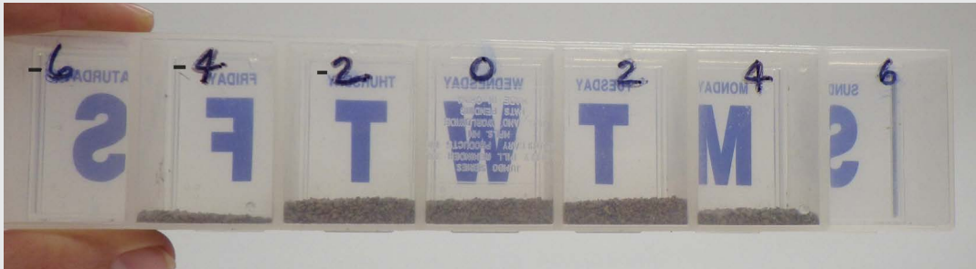
Figure 6. A clear pill box can be used to determine the swath pattern. The numbers correspond to the distance from center (in feet) as in Example A.
