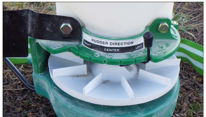
Photo 4. Adjustable rudder positions on a Warren T-7 II spreader.
