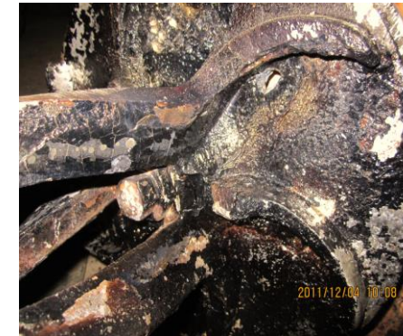
CaCO 3 scale in a MC pump
