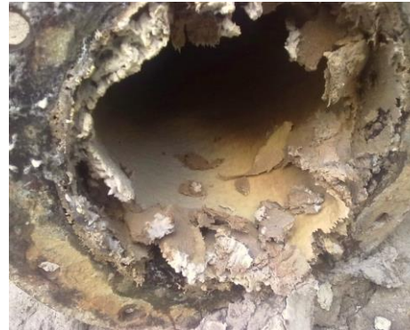
CaCO 3 scale in a EOP pipeline
