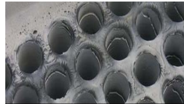
Scale in white liquor heater tubes
