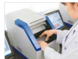
Takara Bio's real-time PCR system, one of the company's products in its PCR-related lineup
