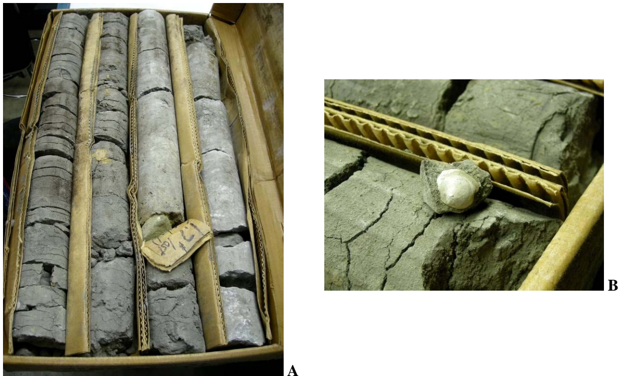
Fig. 7. Photos from Woodruff County Craig Williams core MW No. 6 from 254.8-257.6 m. Core shows lithologic change from the blue gray micaceous silty and clayey sand of the lower McNairy Sand (left side) to the light gray Saratoga Chalk (right side) in A . Bivalve ( B ) shell material is from 255.5 m deep (lower Nacatoch Sand).
