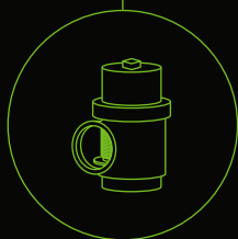
Isolation valves seal high-vacuum chambers from neighboring process elements at different pressure levels.
