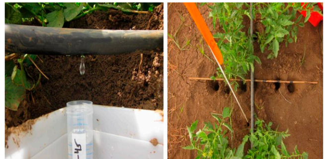
Fig. 12. Sampling of water and soil in field trials for imazapic determination by LCMSMS: (Left) Water sampling of the drip irrigation system. (Right) Soil sampling at vertical distances from the dripper.
