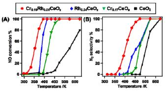
Figure 1. (A) NO conversion and (B)  $N_2$  selectivity for NO reduction with CO on  $Cr_{0.19}Rh_{0.06}CeO_z$ ,  $Rh_{0.04}CeO_z$ ,  $Cr_{0.17}CeO_z$ , and  $CeO_2$ .
