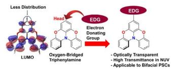
Fig. 1. The molecular design for transparent organic hole-transporting materials.
