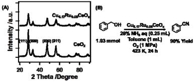
Figure 1 (A) XRD peak pattern of  $Cu_{0.17}Ru_{0.05}CeO_z$ . (B) Catalytic performances for ammoxidation of benzyl alcohol on  $Cu_{0.17}Ru_{0.05}CeO_z$ .
