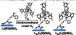
Figure 1. Preparation scheme of surface-attached chiral Tb complex  $(1_{Tb}/L(R/S)/SiO_2)$  by the coordination of  $1_{Tb}$  to  $L(R/S)/SiO_2$ .
