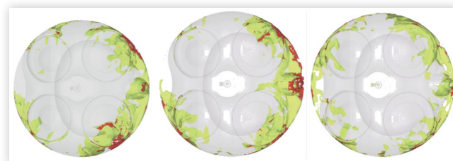
FIGURE 49 Three LES cycles showing flame-front progress and autoignition, from Fontanesi et al. [362].
