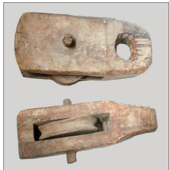
Figure 15. Pulley made of holm oak wood (Etna) (photo T. La Mantia).
