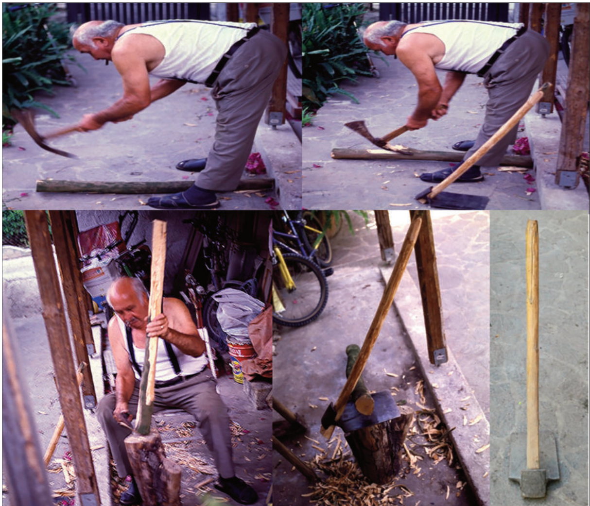
Figure 1. The sequence of images shows (from left to right and from top to bottom) the stages in the construction of a hoe handle by G. La Mantia, father of one of the authors. Sicilian farmers knew how to build various wooden tools on their own (photos T. La Mantia).
