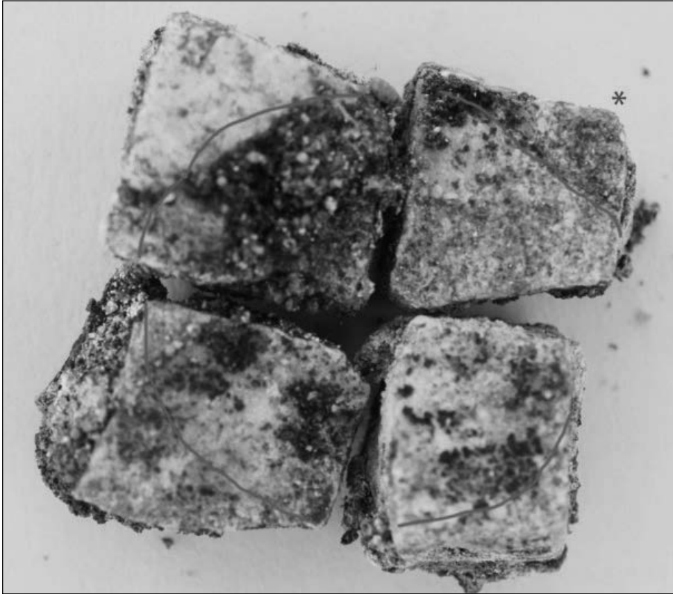
Fig. 12. In situ assays. Mosaic tesserae after treatment with 15% Thyme solution, concentrically diffused with respect to the injection point (highlighted as red line), a lost in pigmentation is clearly recognizable. A vital green colour is still present in the portion not reached (pointed by an asterisk).
