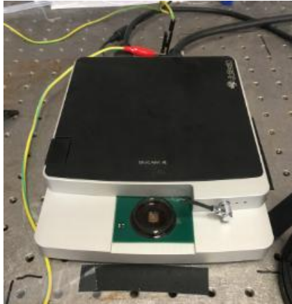
Figure 1.14 | Multielectrode array system. High density MEA (BioCAM X) used for LFP recordings in the GL of mouse cerebellar slices. In green, the CMOS chip with the recording chamber and the microelectrodes.
