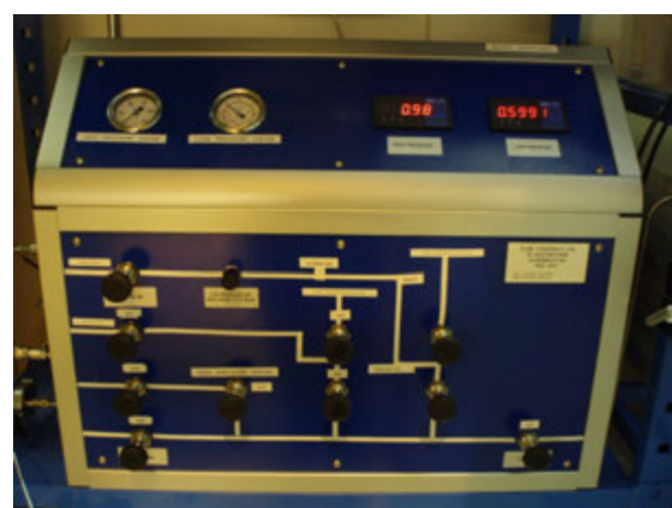
Figure 1: The gas control system, in its specially constructed aluminium support frame, is located outside of the experimental hutch.
