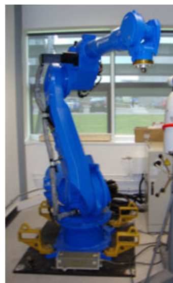
Figure 1: Robot arm at beamline I13. The device replaces the traditional diffractometer, holding the future EXCALIBUR detector at large distance for coherent X-ray diffraction experiments.
