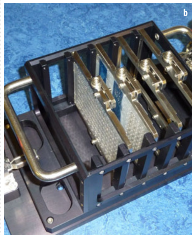
Figure 1: a) In situ set up on the I24 microfocus beamline. The plate is positioned into the beam using a modified goniometer system. b) Rack from which the I03 ACTOR sample changer picks up crystallisation plates and mounts them to the goniometer. c) In situ set up on I04-1 using the CATS sample changer to position plates in the X-ray beam.
