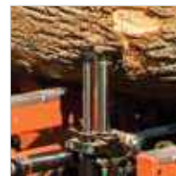
Hydraulic Clamp, Two Hydraulic Side Supports & Two Manual Side Supports Secure and stabilize the log.
