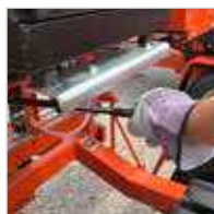
Blade Guide Arm Easily move blade guide arm from operators position to increase accuracy.
