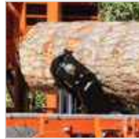
Hydraulic Bi-directional Chain Log Turner For maximum log control.
