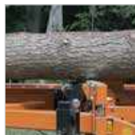
Hydraulic Toeboards For precise log leveling.
