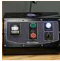
Electrical Auto Feed Control Box Auto/Manual index switch and tooth counter
