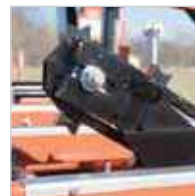
Hydraulic Bi-directional Chain Log Turner Industrial #2080 ANSI chain for maximum log turning
