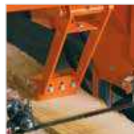
Auto Board Return Arm and Table Assists with off-bearing boards. 610 mm x 610 mm (2' x 2') table attached.
