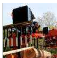
Deluxe Board Return Arm and Table Assists with off-bearing. 914 mm x 1,5 m (3' x 5') table Only available with electric DCS Control (RD).
