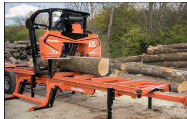
7 Bedrails with Stainless Steel Sleeves For optimum log support
