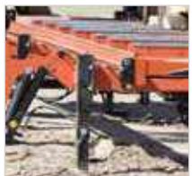
Set of 6 Heavy Duty Fine-Adjust Outriggers For mill stability and bed leveling
