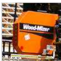
Hinged Blade Wheel Covers For quick blade change.
