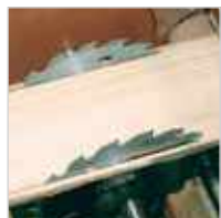
One fixed and one movable blade edge both sides of your board in one pass, saving you time.
