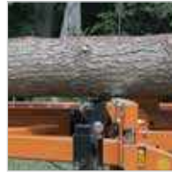
Hydraulic Toeboards For precise log leveling.
