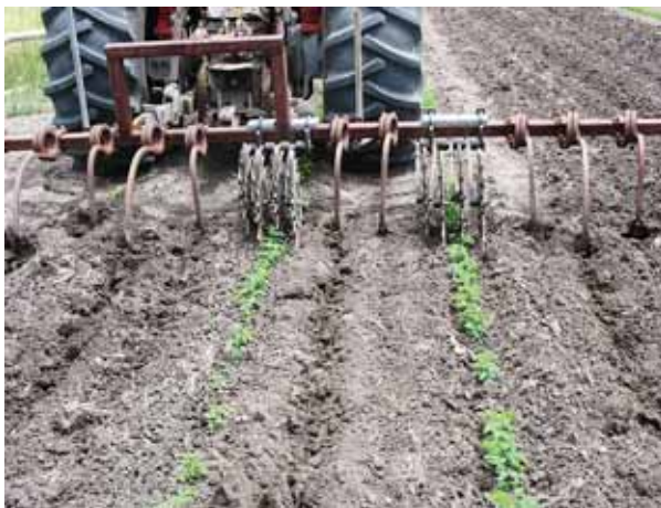
Above and below. Mechanical weed control with Yetter wheels over the rows and scufflers between.
