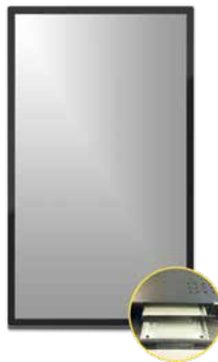
Swappable dual HDD/SSD slots for easy updates
