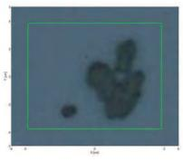
Figure 6 Microscope image of a TiO2 particle on a silicon substrate
