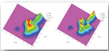
Figure 7 Raman imaging of a TiO2 particle on a silicon substrate (Intensity profile of the TiO2 peak height) (left; by ordinary confocal system ('a' of Figure 5), right; the JASCO DSF system ('b' of Figure 5)
