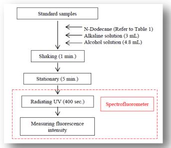
Figure 2 Flow chart of analysis procedure
