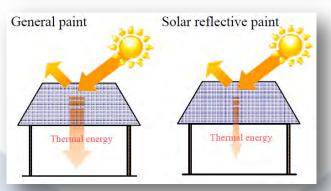
Figure 2 Conduction of solar thermal energy
