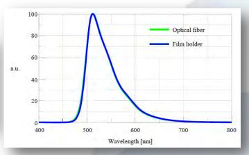
Figure 2 Peak normalized fluorescence spectrum of the yellow card
