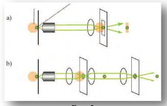
Figure 5 (a) standard confocal optics with pinhole aperture (b) JASCO DSF confocal optics
