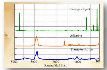
Figure 2 Spectrum for each layer
