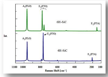
Figure 1 Raman Spectra of 6H-SiC and 4H-SiC
