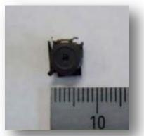
1-mm-diameter mobile-phone camera lens
