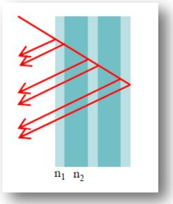
Figure 1 Diagram of the dielectric multi-layer mirror n<sub>1</sub>: high refractive index n<sub>2</sub>: low refractive index
