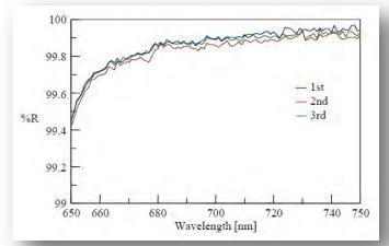
Figure 4 Absolute reflectance spectra of the dielectric multi-layer mirror at around 100%R
