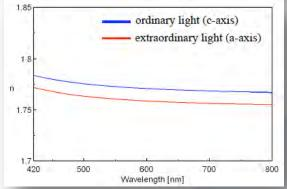
**Figure 2** Wavelength dispersion of refractive index of monocrystalline sapphire above: by using [UVVis K-K Conversion] Program below: by using [Multi-layer Analysis] Program
