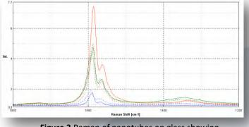
Figure 3 Raman of nanotubes on glass showing the G/D region
