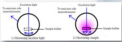
Figure 2 Diagram of integrating sphere for measuring incident light and measuring sample
