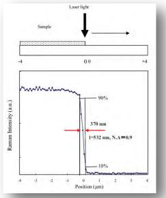
Figure 3 Measured spatial resolution in NRS-5000/7000 (532 nm laser , objective lens 100x) (upper – illustration for measurement of silicon sharp edge; lower – Raman intensity profile of silicon peak)
