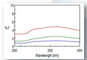
Figure 2 Transmittance spectrum of each sample Red line: T shirt Blue line: Sports shirt Green line: Arm cover
