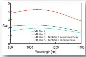
Figure 3 Absorbance spectra of ND filter
