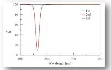
Figure 3 Absolute reflectance spectra of the dielectric multi-layer mirror
