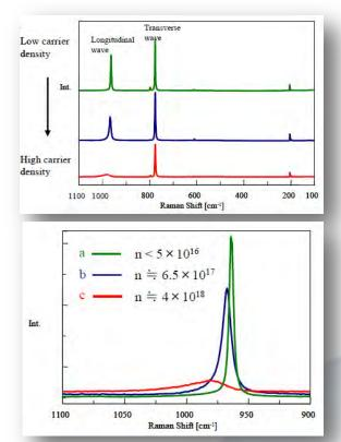
Figure 3 Change of Raman spectrum of 4H-SiC due to carrier - concentration(A), zoomed one (B)
