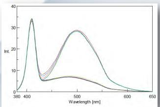
Figure 6 Spectra of conc. 0 and 1 % coumarin solution (5 spectra each)
