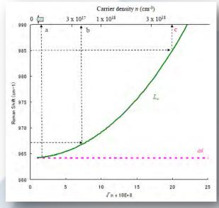
Figure 4 Carrier concentration calculation from central wavenumber
