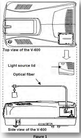
V-600 series spectrophotometer with the external source fiber optic interface
