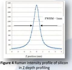
(532 nm laser, objective lens 100x, N.A=0.9)
