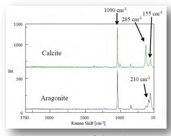
Figure 3 Raman spectrum of calcite and aragonite
