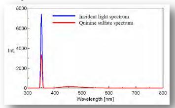
Figure 4 Emission spectrum of quinine sulfate
