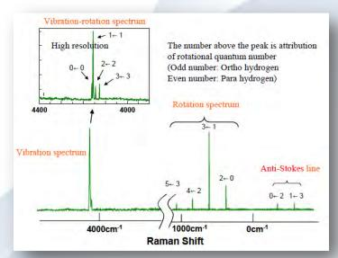
Figure 2 Raman spectrum of hydrogen gas
