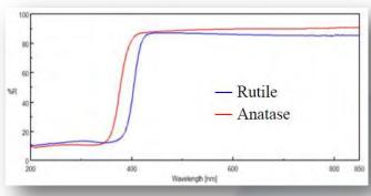
Diffuse transmittance spectrum for TiO2
