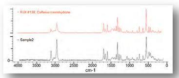
Figure 3 - The result of non-opening measurement of solid sample in a brown bottle by using macro measurement unit (Top: Database, Bottom: Measurement result)
