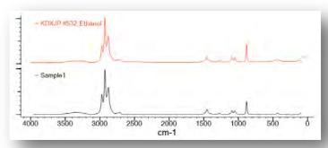
Figure 2 - The result of non-opening measurement of liquid sample by using macro measurement unit (Top: Database, Bottom: Measurement result)
