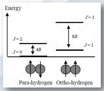
Figure 3 energy level of ortho-para hydrogen
