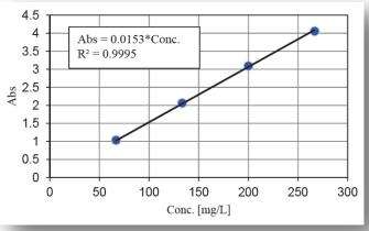
Figure 2 Calibration curve at 526 nm
