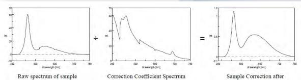
Sample Correction after the Spectrum Correction
