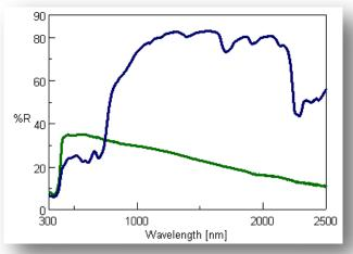
Figure 5 Diffuse reflectance spectra of solar reflective paint material and general water paint
