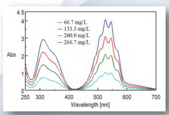
Figure 1 Absorbance spectrum KMnO4 solution
