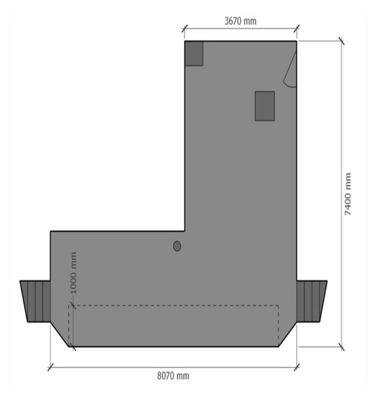
Dotted line indicates 'uncovered' section. The rest is fully under the stage at a height of 2400mm
