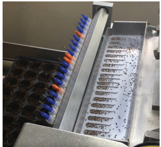
Figure 6. Semi-automated machine seeding Paronychia erecta into propagation flats within a commercial propagation facility in Pensacola, Florida.
