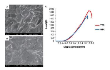
Figure 2. Scanning electron microscopy (SEM) imaging and load-displacement curves of the traditional titanium cage (TTC) and helical-shaped titanium cage (HTC). SEM analysis of the TTC (A) and HTC (B) showed the rough surfaces of both samples. (C) Load-displacement curves of the TTC and HTC revealed the status of the compressive strength of TTC and HTC.
