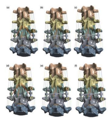
Fig. 2 Finite element models of lumbar fusion utilizing various designs of tethering device: (a) PLIF with split tethering, (b) PLIF with one-way tethering, (c) PLIF with two-way tethering, (d) PLF with split tethering, (e) PLF with one-way tethering, (f) PLIF with two-way tethering
