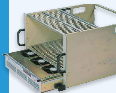
CAMAC bin with fan tray removed
