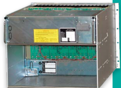
6U cPCI 6021 Crate outfitted with four 5-slot 6U backplanes rear view
