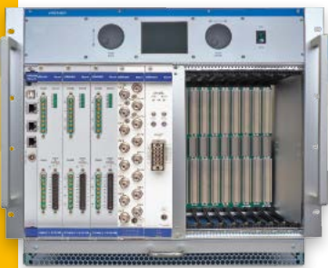
MPOD-9 slot VME64x mixed crate with air filter
