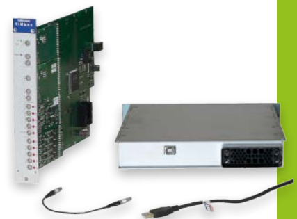
Left: open NIMbox (custom version) with DL706 main board and 4 submodules plugged in. Right: NIMbox rear side with USB port and NIM connector
