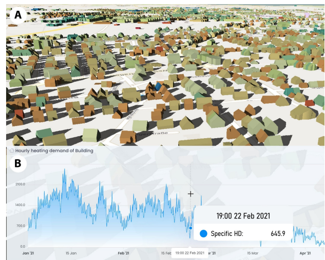
Figure 8. A visualization in the EnSysLE UDT application illustrating A: 3D city models styled according to the calculated specific space heating demand (kWh/m 2 /yr), B: the pop-up window showing hourly heating demand (kW) of the selected building.
