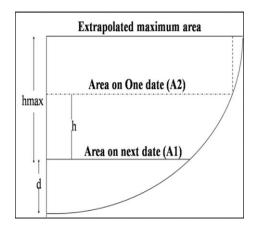
Fig. 2. Modified Trapezoidal Method Line diagram (source: (Shukla et al., 2017)
