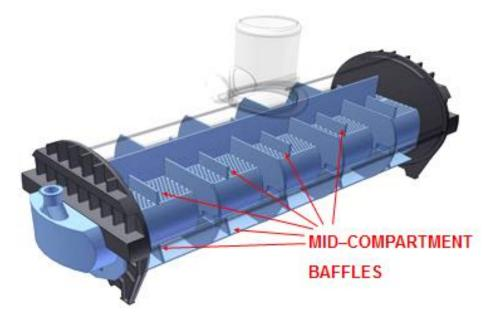
Figure 4: Mid-compartment flow baffles
