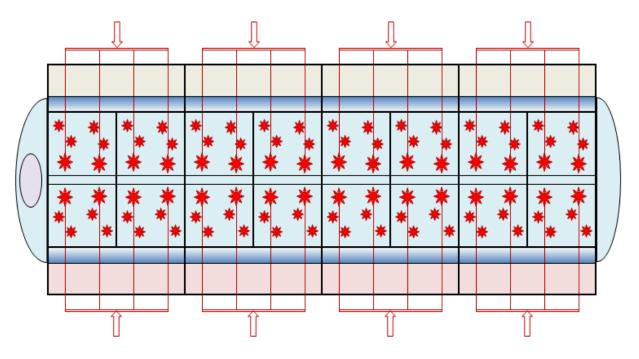
Figure 3b. Feed and jigger distribution beneath calandria
