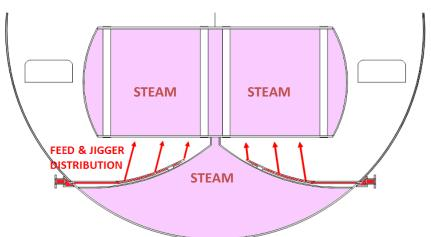
Figure 3a:Feeds and Jigger steam injected below massecuite
