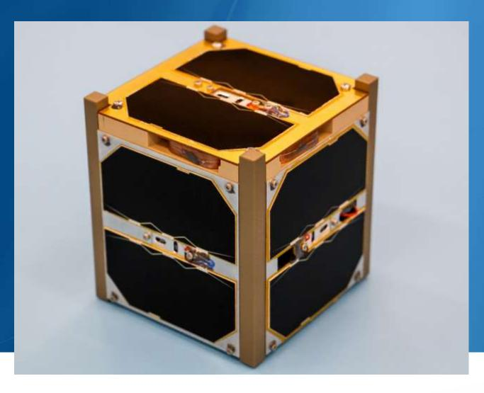
A "standard 1U" CubeSat has a volume of one liter - 10 cm cube and a mass of 1 kg, orbiting at 300-600 km circular orbit, 1W transmitter on 145 or 435 MHz amateursatellite service band. It's used for academic education, research and technology validation applications but also for complex science and governmental use
