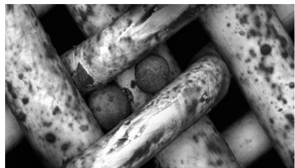
Figure 5 - Microscope photograph of cat fines entrapped in the mesh of a fuel filter
