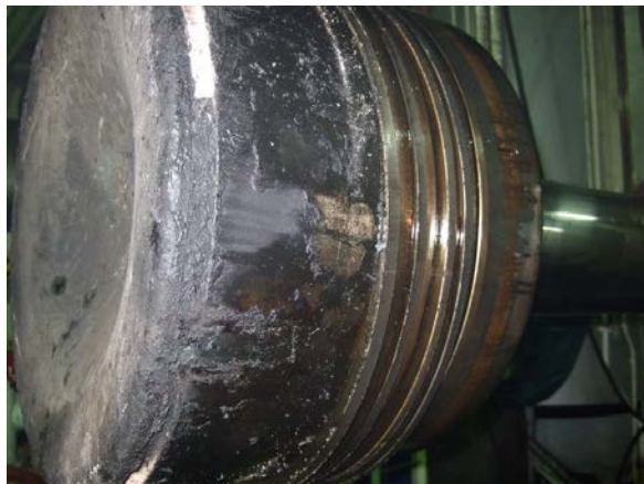
No. 4 Unit piston – note broken 2nd ring
