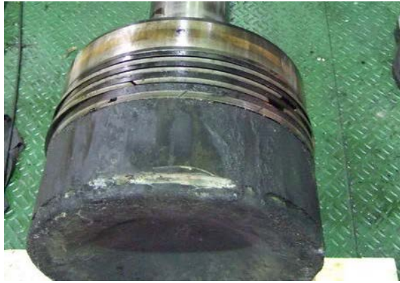
No. 1 Unit ME Piston (after only 240 running hours)
