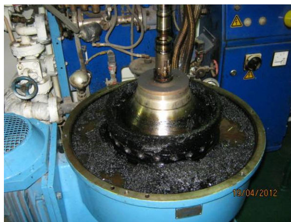
Figure 16 - excess sludge build up in the purifier casing
