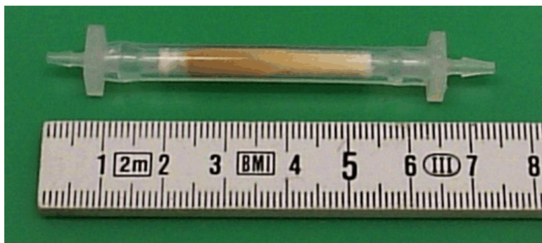
Fig. 4.89.2: Institute for Transuranium Elements (ITU) Standard ^{225}\text{Ac}/^{213}\text{Bi} Radionuclide Generator. Image kindly provided by Dr. Alfred Morgenstern, European Commission, Joint Research Centre – Institute for Transuranium Elements, Karlsruhe, Germany.
