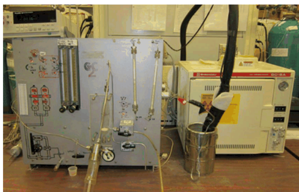
Fig. 4.28.2: Shimadzu GC-8A Gas Chromatograph (GC) with an Electron-Capture Detector (ECD). (Image Source: The Reston Chlorofluorocarbon Laboratory, U.S. Geological Survey) [233, 234].
