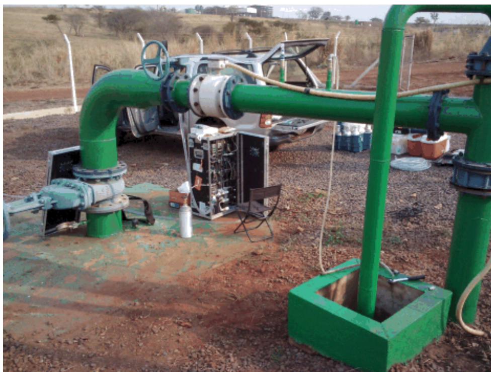
Fig. 4.36.1: ^{81}\text{Kr} has been used to date the groundwater being discharged from springs and wells. The photo shows collection of a ^{81}\text{Kr} sample from an artesian well in Farafra Oasis, Egypt [289]. (Photo Source: N. C. Sturchio, University of Delaware, Delaware, USA).
