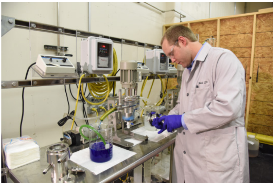
Fig. 4.89.1: The Medical Actinium for Therapeutic Treatment (MATT) is a separations process that recovers ^{225}\text{Ac} from unused nuclear fuel so the isotope can be used in cancer treatment and research. (Image Source: Idaho National Laboratory) [588].
