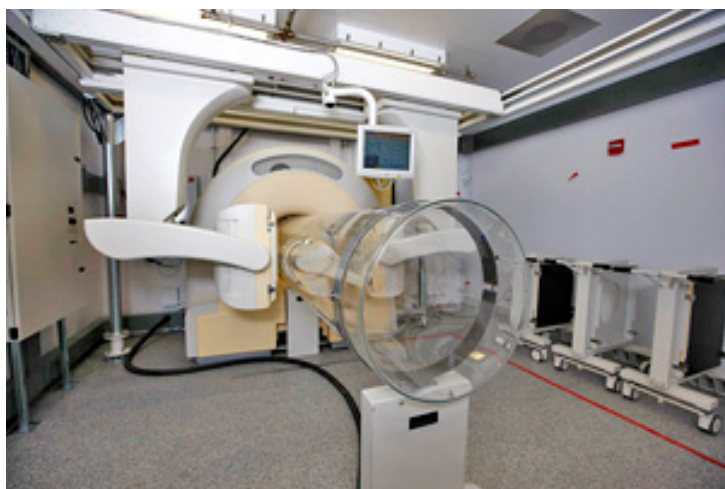
Fig. 4.43.1: Single-photon emission computed tomography (SPECT CT) machine. (Image source National Institute of Allergy and Infectious Diseases (NIAID) and National Institutes of Health) [325].
