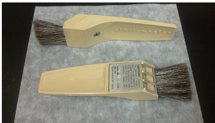
Fig. 4.84.1: Staticmaster™ Alpha Ionizing Brushes for cleaning optical surfaces and photographic films have a soft, non-abrasive brush and a ^{210}\text{Po} cartridge. (Photo Source: Reston Stable Isotope Laboratory of the U.S. Geological Survey) [564].
