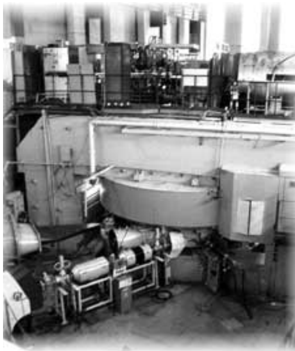
Fig. 4.116.1: Photo of the heavy ion cyclotron U-400 at JINR in which livermorium was synthesized. (Photo Source: Lawrence Livermore National Laboratory) [675].
