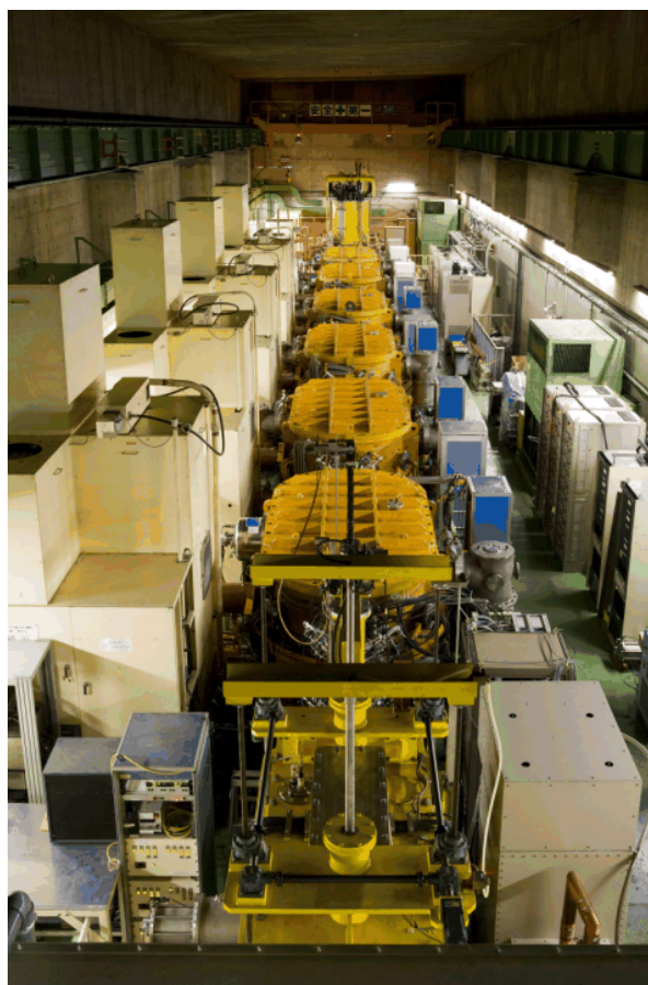
Fig. 4.113.1: RILAC (RIKEN linear accelerator) used to synthesize nihonium (kindly provided by RIKEN).
