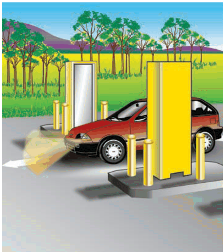
Fig. 4.2.1: Radiation detectors are installed in many areas to screen people, vehicles, and cargo for radioactive materials. ^3\text{He} detectors are sensitive to thermal neutrons and are used to detect isotopes of uranium and plutonium that might be used in nuclear weapons, along with other sources that produce neutrons by radioactive decay . (Image Source: U.S. Government Accountability Office) [33].
