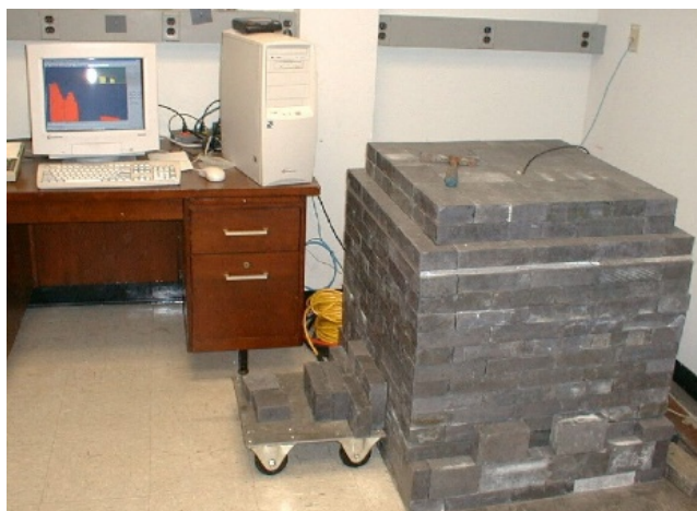
Fig. 4.63.2: ^{152}\text{Eu} is used as a reference source for calibrating gamma-ray spectrometer systems like the one pictured here. (Photo Source: Snyder and Duval, 2003. U.S. Geological Survey Open-File Report 03-029) [450].
