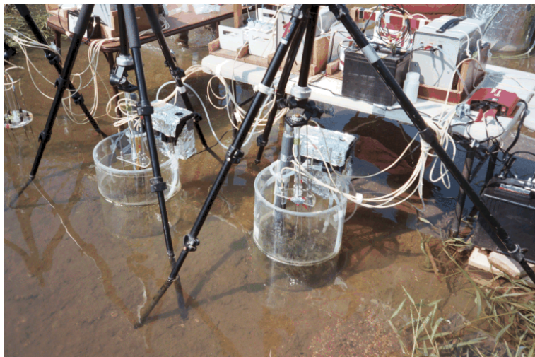
Fig. 4.7.2: Tracer experiments with the stable isotope ^{15}\text{N} have been used to track excess dissolved nitrate in groundwater and streams and to determine to what extent the dissolved nitrate is removed by natural processes, such as conversion to harmless \text{N}_2 gas before entering nitrogen-sensitive ecosystems [83]. (Photo Source: Böhlke, J.K., U.S. Geological Survey).
