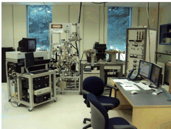
Fig. 4.18.2: The U. S. Geological Survey ^{40}\text{Ar}/^{39}\text{Ar} geochronology laboratory in Denver, Colorado uses a custom-built argon extraction line connected to a Mass Analyzer Products (MAP) 215-50 mass spectrometer with a differentially pumped dual laser setup. (U.S. Geological Survey ^{40}\text{Ar}/^{39}\text{Ar} Geochronology Laboratory) [175].
