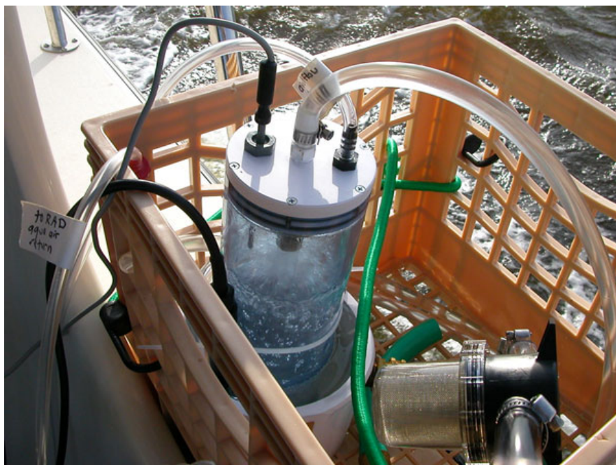
Fig. 4.86.1: Air-water equilibrator, which strips radon out of water and into the gas phase so it can be used as a groundwater tracer . (Photo Source: John Crusius, U.S. Geological Survey) [573].
