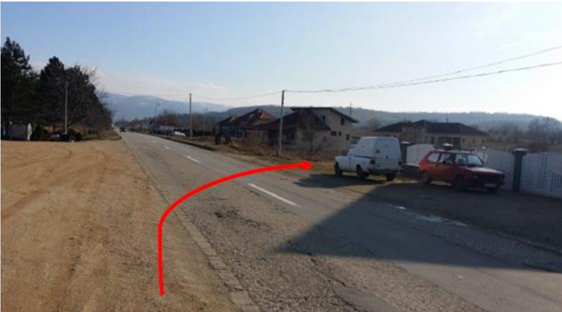
Figure 44: Access roads network – widening turn required
