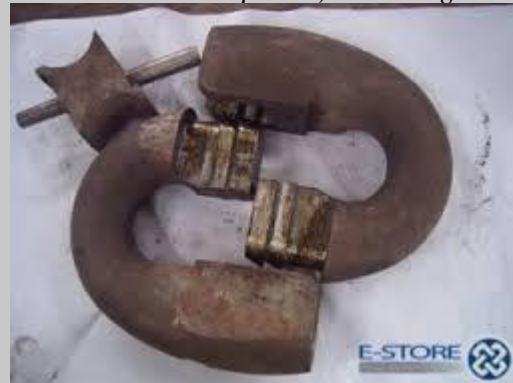
Kenter shackle on deck and open it with pin and hammer.
