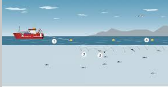
1. the main line 2. baited hooks on branching lines also known as snoods 3. bycatch can be a problem with longlining 4. floats
