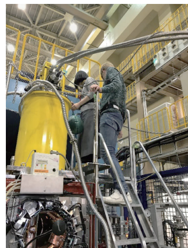
Figure 3. Users from Toyota CRDL and KTH Sweden are preparing the sample mounted in a cryo-furnace.
