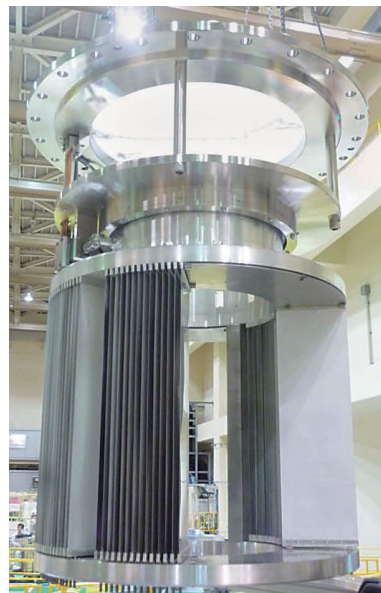
Figure 1. Radial collimator installed at NOVA.
