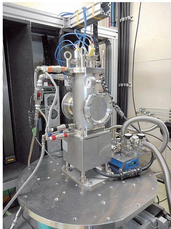
Figure 1. Furnace for small-angle scattering and neutron reflectivity measurement.
