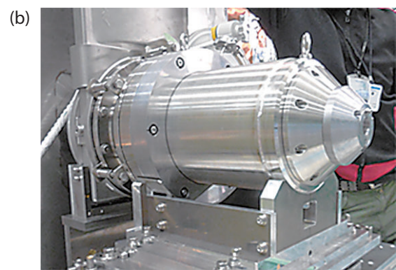
Figure 2. Beam collimator: (a) design (b) its picture patteim-age obtained by profile monitor.
