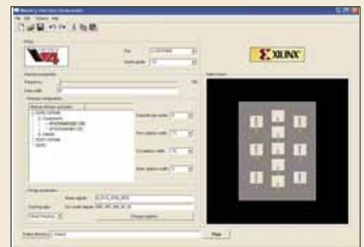
Figure 2 – Memory interface generator
