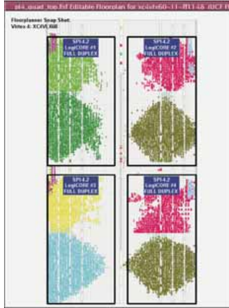
Figure 3 – Illustration of four SPI-4.2 LogiCORE IP implemented on a Virtex-4 XC4VLX60 device
