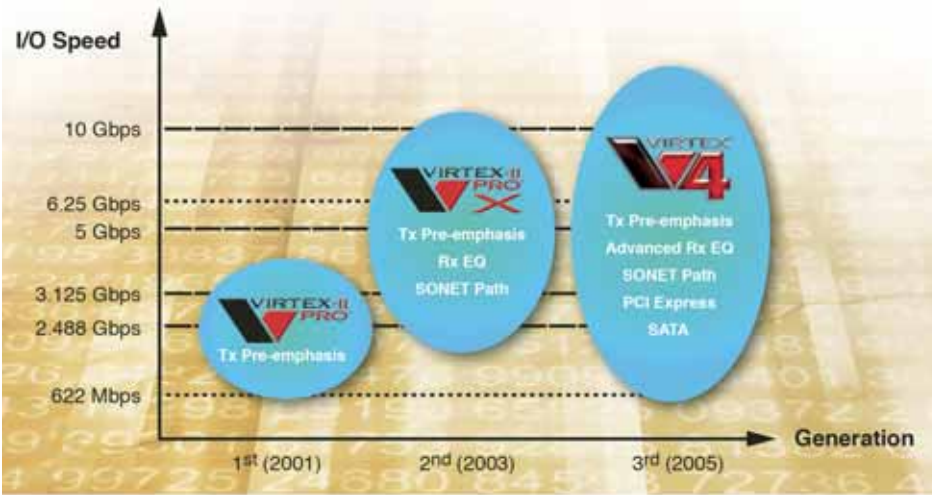
Figure 1 – Evolution of the RocketIO transceiver
