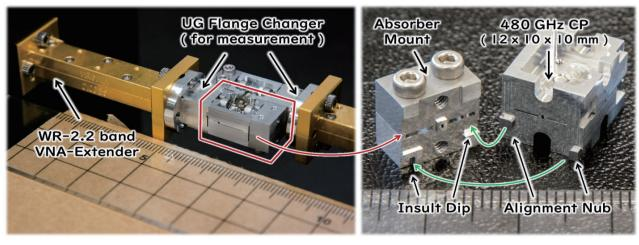
Photographs of the developed 480 GHz Circular Polarizer (CP)
