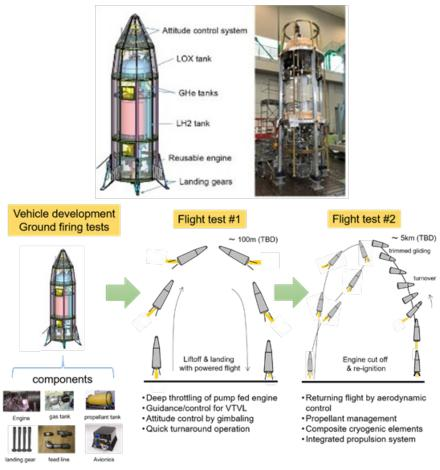
Flight demonstrations by reusable rocket vehicle RV-X.
