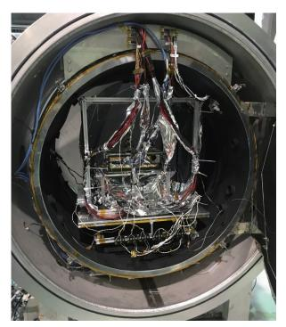
Thermal vacuum test for the engineering model for EQUULEUS
