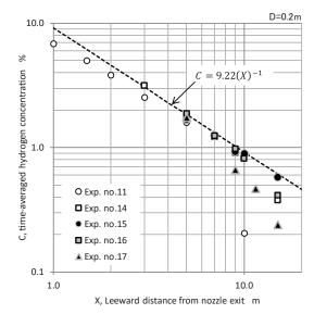
The 1% hydrogen concentration distance was necessary to extend 2 m as compared with the conventional safety standard.
