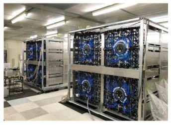
Fig.2 Pair of 15.8-kW X-band SSPA #1 and #2 output section.
