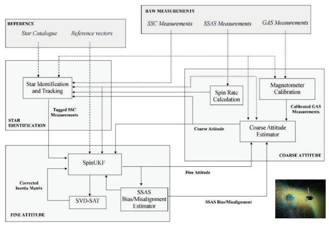
On ground attitude determination system with SpinUKF for the ARASE (ERG) satellite
