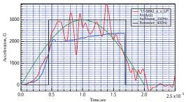
Fig.3A Impact shock acceleration (Approx. 1 ms) of the Urethane at a speed of 30 m/s onto the hard target was compared with the sine-wave and rectangular wave.
