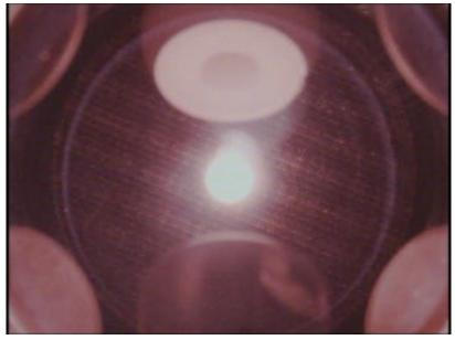
A molten erbium-oxide sample levitated in the ISS-ELF.
