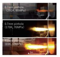
Pictures of hydrogen combustion flame under various temperature conditions.
