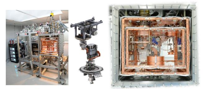
Setup of the Cryostat 1 experiment at CEA. (Left) The cryostat with JT coolers and control electronics. (Middle) Schematics of the coolers. The hybrid coolers located at the center, 2K-JT are connected from the top and 4K-JT from the bottom. (Right) Close up of the actual cryostat. A GSE cooler is at the left-top.
