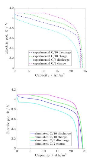
Fig.2 Battery voltage vs capacity. The top graph shows data from ISAS. The bottom graph is simulation data from DLR
