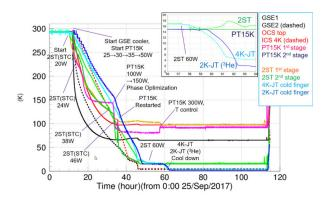
Temperatures of several tests from 300 K to < 2K. Data taken at CEA (2017/9/25~).
