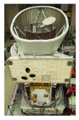
MMO during the environmental test performed at ESA/ESTEC. Sine vibration test for the MCS (configuration of BepiColombo during cruise). The MCS is on the shaker for lateral vibration. The bottom square part of MCS is the MTM (Electrical propulsion module). The middle rectangular part is the MPO (Mercury Planetary Orbiter). The MMO is located at the top of the MCS. The white cone surrounding the MMO is the sunshield.
