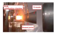
Fig.2 Image of the combustion test.
