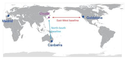
Ground stations were used for this measurement. By using the Japanese Usuda Station in combination with the DSN facilities, two-dimensional simultaneous Delta-DOR measurement became possible for the first time.
