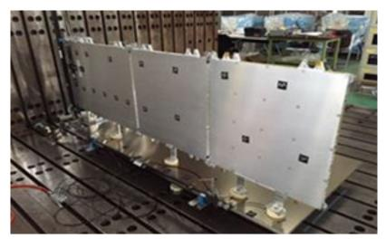
Deployable SAR Antenna Assembly Consists of Planar Slot Array Panels.
