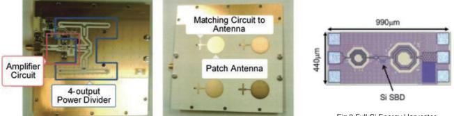
Fig.1 Active Integrated Antenna Array
