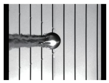
Fig.3 Shape of the formed impact head observed in the ground test. It was almost identical to the result of the computational simulation. The speed of the impact head was more than 2 km/s.
