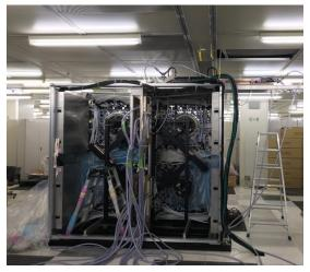
Fig.1 Exterior of input section of a 15.8-kW X-band SSPA #1 assembly.
