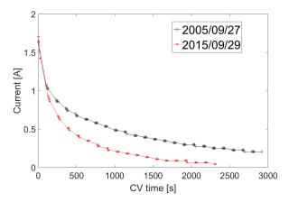
Fig.1 Decay curves of the REIMEI onboard battery in 2005 (immediately after launch) and 2015 (after 60,000 charge/ discharge cycles).
