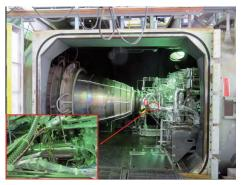
Capacitive void fraction sensor for LE-5B-3 ground tests
