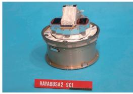
Fig.1 Small Carry-on Impactor. Weight is Approx.14kg.
