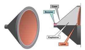
Fig.2 Developed shaped charge for Hayabusa2 impact mission. It includes 4.7 kg HMX-based polymer-bonded explosive.
