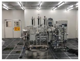
New clean chamber installed in a new clean room for Hayabusa2 samples.
