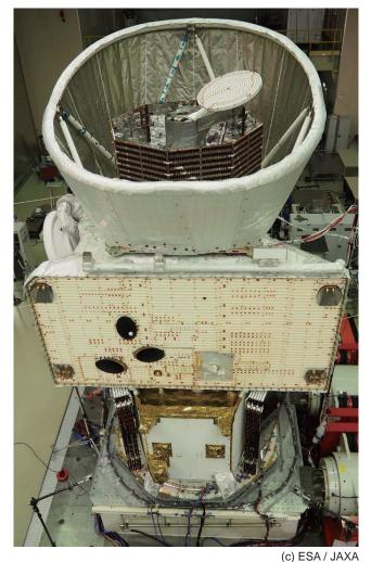
MCS (Mercury Cruise System) vibration test at ESTEC.
