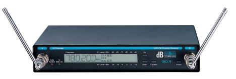
Multi-channel-Applications The receiver in a 9.5" metal casing provides information on all the essential operating parameters, such as operating frequency, HF and audio level and also the battery status of the transmitter, through its large illuminated display. The antennae are mounted on the front and can be removed allowing them to be repositioned or permitting the use of the optional active antenna splitter AS6 in multi-channel applications.
