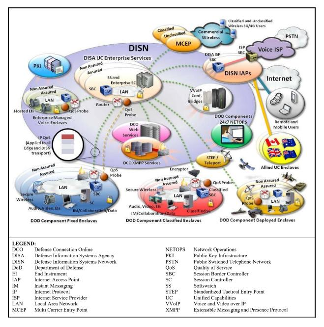
Figure 2-1. Notional DoDIN Network Architecture
