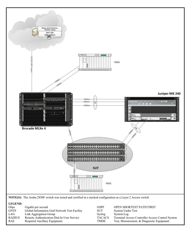
Figure 2-3. SUT Stacked Architecture with Heterogeneous Test Configuration
