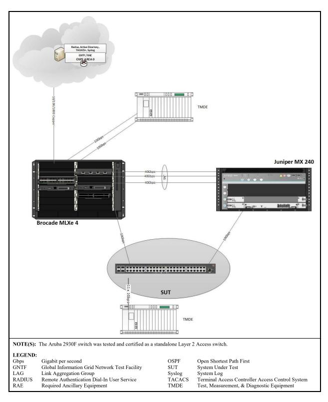
Figure 2-2. SUT Single Switch Architecture with Heterogeneous Test Configuration
