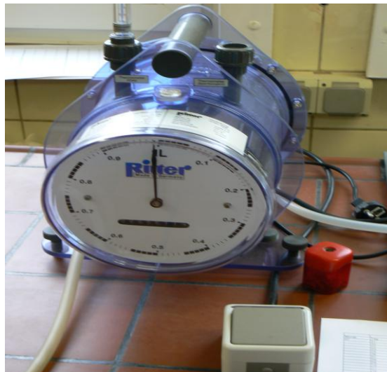
Fig. 3.5: Ritter wet gas meter used in biogas laboratory in Raischholzhausen
