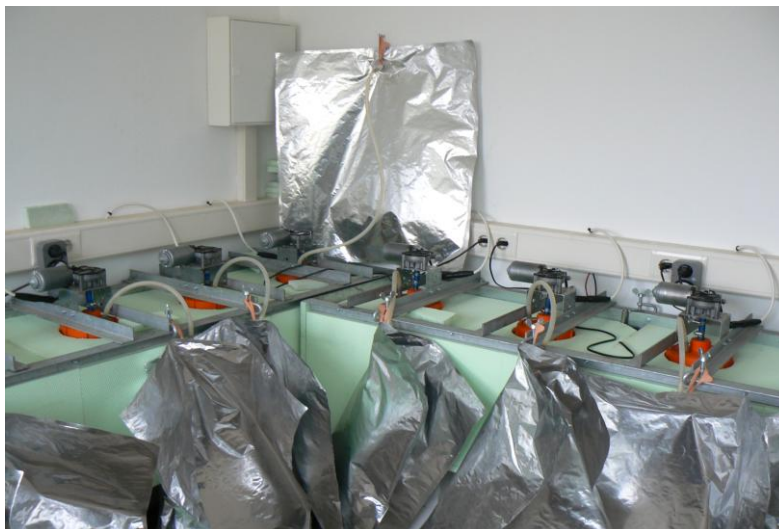
Fig. 3.4: Laboratory mesophilic digesters in the research station Rauschholzhausen
