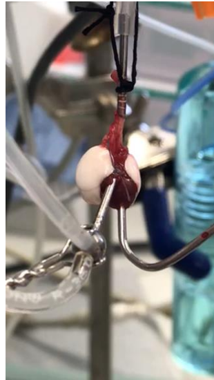
Figure 6. The isolated perfused and ventilated mouse lung setup
