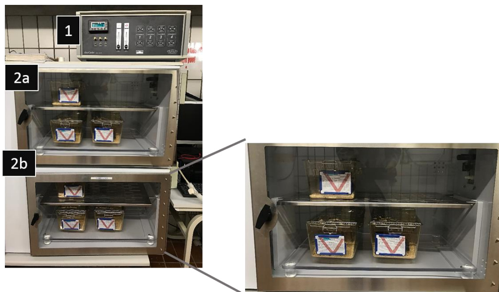
Figure 8. Hypoxic and normoxic incubation chambers.
