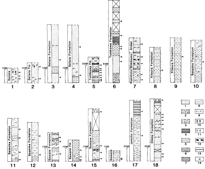
Fig. 5. Columnar sections for Omma-Manganji sections 1-18. Datum is base of section, and sections 7-12 are schematic representations. Lithological symbols: 1-sand, 2-coarse sand, 3-calcareous sand, 4-clay, 5-silt, 6-conglomerate, 7-diatomite, 8-tuff, 9-shell, 10-gastropods, 11-burrows, 12-wood, 13-unconformity, 14-ostracod sample horizon.
