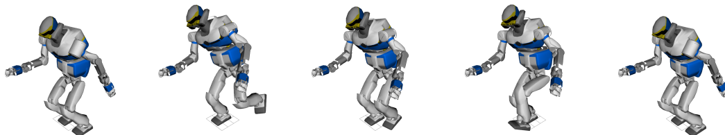
Figure 1: Snapshots from a whole-body motion planning scenario with the HRP-2 humanoid robot. High-level nonlinear tasks can easily be added. Here, the robot achieves a kicking motion with a minimum velocity of 1m/s, while keeping its CoM above its right foot, keeping its right hand fixed in position and orientation under joint position and speed limits. Computation took less than 700 ms with a GeForce GTX Titan Black GPU for that 5-second motion. The optimization problem consists in 336 variables and 1960 constraints.
