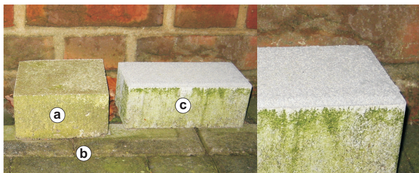
Figure 7.3: Staining of concrete paving blocks caused by algae growth: a) untreated sample, b) paving of standard paving blocks, and c) paving block containing \text{TiO}_2 in the functional top layer.
