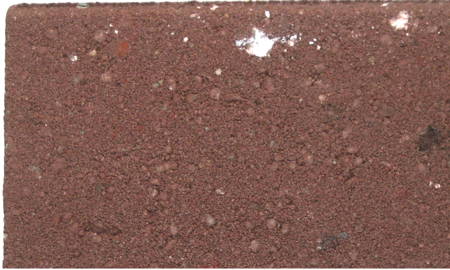
Figure 8.4: Agglomerates of \text{TiO}_2 formed on the surface of a concrete paving block.
