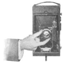
FIGURE 14. Reducing shutter spring tension.
