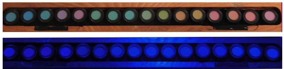
Figure 3 Arrangement of the D15 Under the Blue Light and the Same Arrangement Under Daylight
