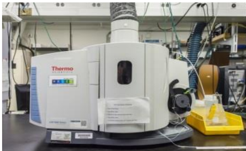
Fig. 3: Inductively Coupled Plasma (ICP) Atomic Emission Spectrometer.
