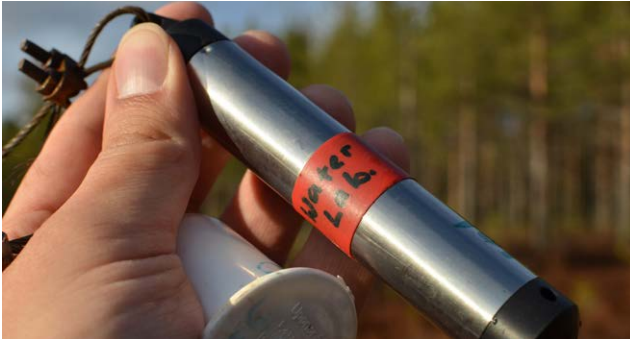
A data logger for monitoring water level fluctuations in restored mires. Photo: Lauri Ikkala.
