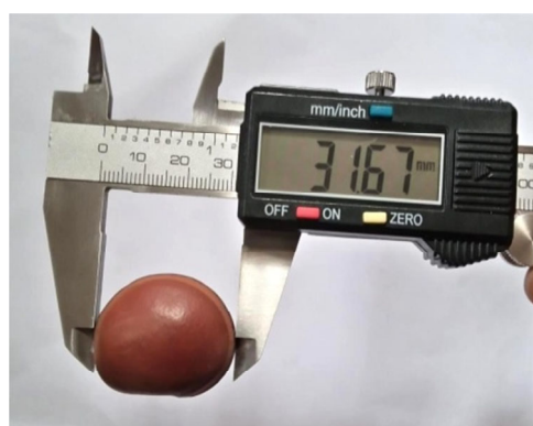
Figure 1 - (a) Representation of the three perpendicular dimensions of Dioclea reflexa seed. (b) Dimensional seed measurement with Vernier caliper
