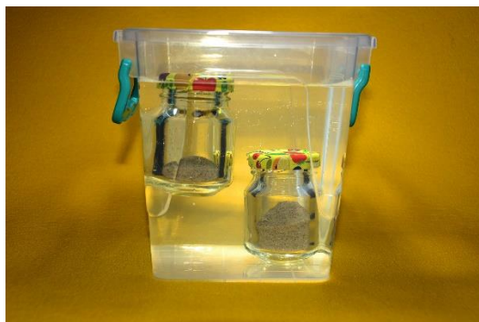
Fig. 2. The level of immersion of two objects with different mass but with the same volume.
