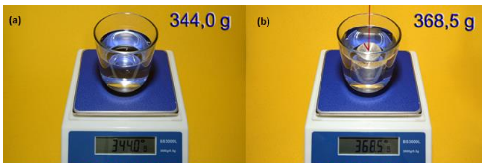
Fig. 5. (a) Mass of the beaker of water; (b) Mass of the beaker of water with cylindrical object inside
