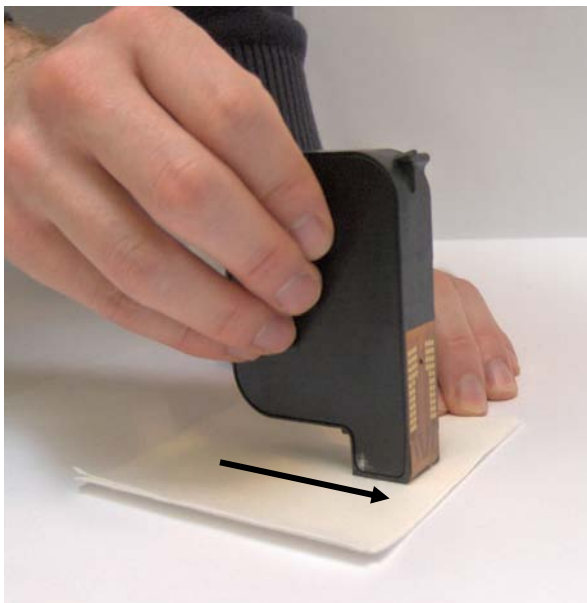
Figure 50: Cleaning the nozzle plate
