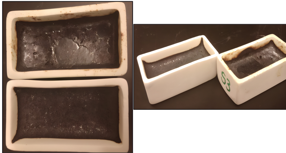
Figure 3.3: Behaviour of the MgO Crucible During Pre-melting of the Slag
